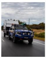
the next thing to consider is your tow ball weight. As a rule of thumb, you should aim to keep your tow ball weight within 10% of Aggregate Trailer Mass (ATM). Going above or below this figure leads to two different scenarios, both potentially catastrophic.
